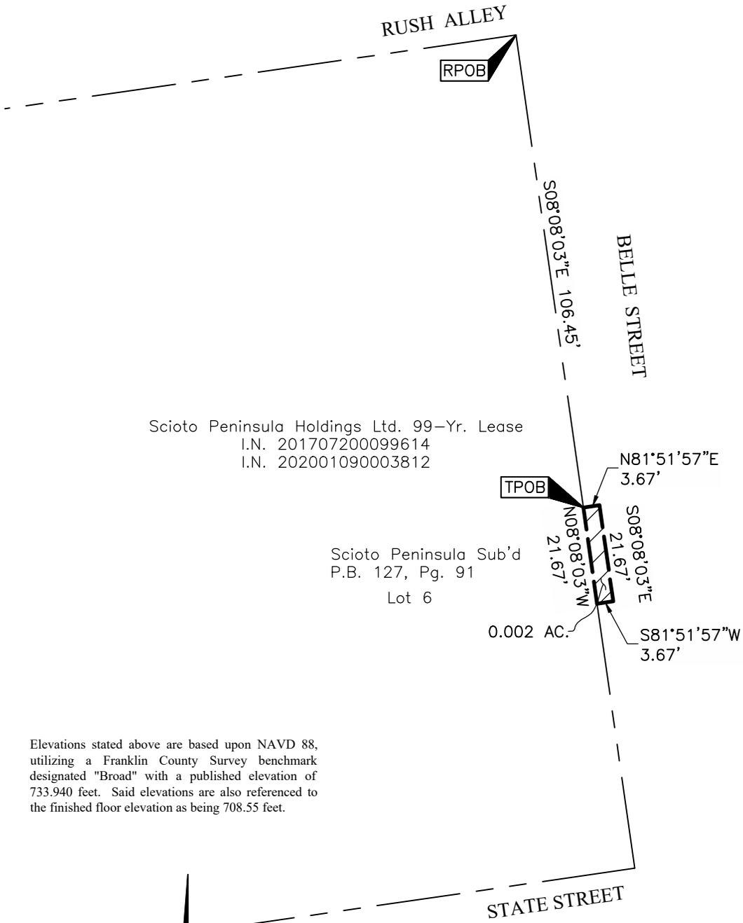
Elevations stated above are based upon NAVD 88, utilizing a Franklin County Survey benchmark designated "Broad" with a published elevation of 733.940 feet. Said elevations are also referenced to the finished floor elevation as being 708.55 feet.
