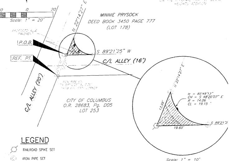
IRON PIPES SET ARE 3/4" I.D. 30" LONG IRON PIPE WITH A YELLOW CAP STAMPED (RAAB ."P.S. 7863)
