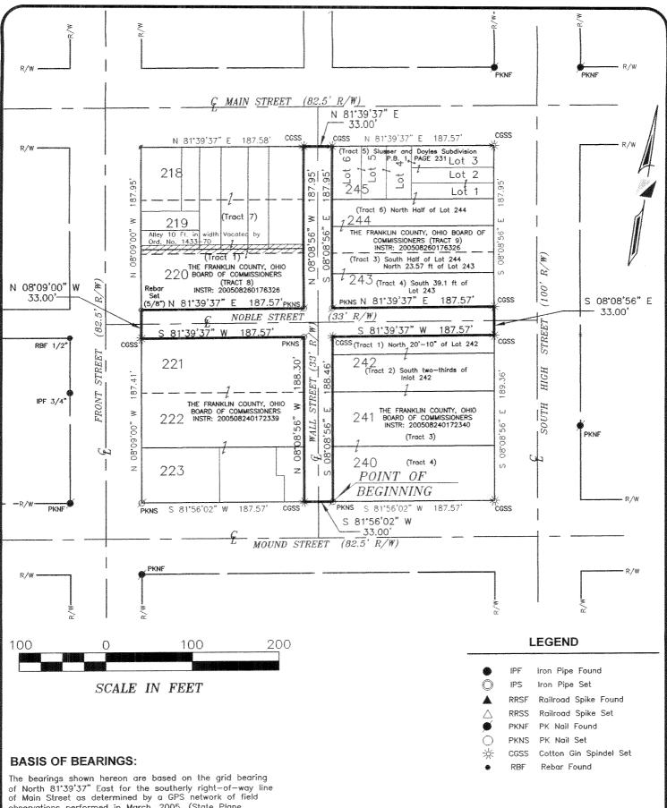
The bearings shown hereon are based on the grid bearing of North 81'39'37" East for the southerly right-of-way line of Main Street as determined by a GPS network of field observations performed in March, 2005, (State Plane Coordinate System, South Zone, 1995 Adjustment-CORS).
