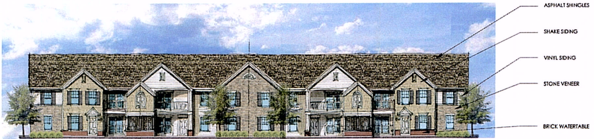
TYPICAL 2-STORY VISTA BUILDING ELEVATION SCALE: N.T.S.
