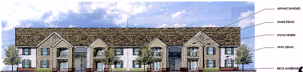
TYPICAL 2-STORY BREEZEWAY BUILDING ELEVATION SCALE: N.T.S.
