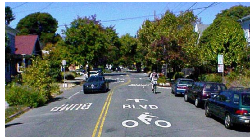
One of many possible treatments to create a bike boulevard.
