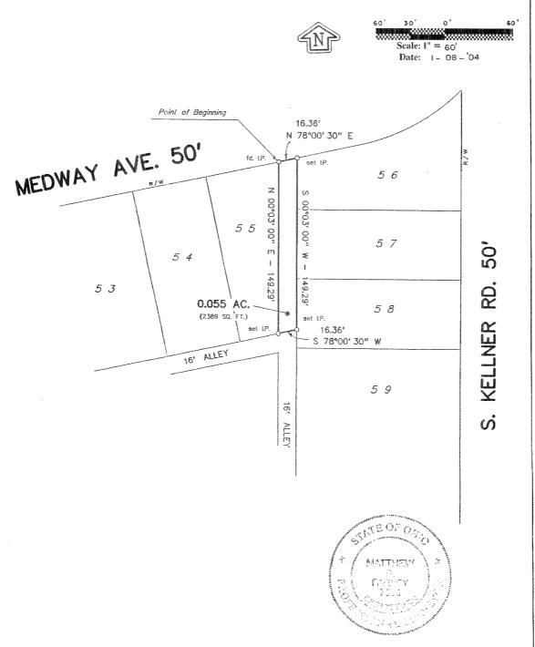
We hereby certify that the foregoing Boundary Survey was prepared from actual field measurements in accordance with Chapter 4733-37 Ohio Administrative Code. Iron pins set are 30"x1" O.D. with an orange plastic plug inscribed "P.S. 6579", unless otherwise noted. Basis of bearing is the centerline of South Kellner Road held as South 00 degrees 03 minutes 00 seconds West, per Plat Book 16, Page 21
