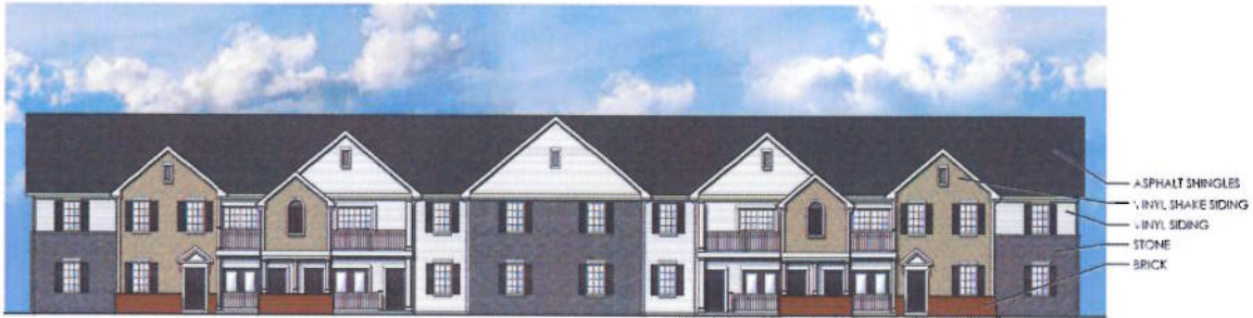
① BUILDINGS 2 & 4 ELEVATION SCALE: 1" = 10'
