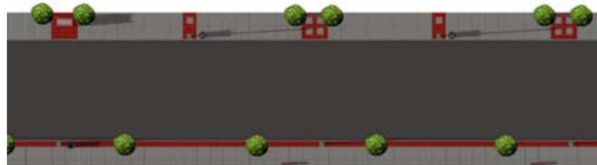
Proposed Main improvement elements within the city right-of-way include brick paving, pedestrian lights, trees, trash receptacles and bus shelters. Source: Milo-Grogan Capital Improvement Plan by Columbus Neighborhood Design Assistance Center.
