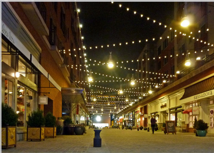
The sidewalk and street are level to allow for varying transit modes.
