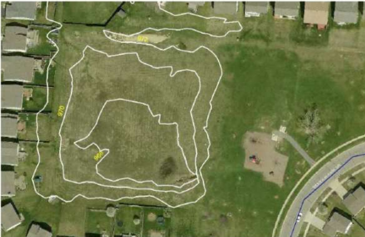
Figure 4: Crawford Farms Park stormwater basin with elevations in feet above sea level contours marked
