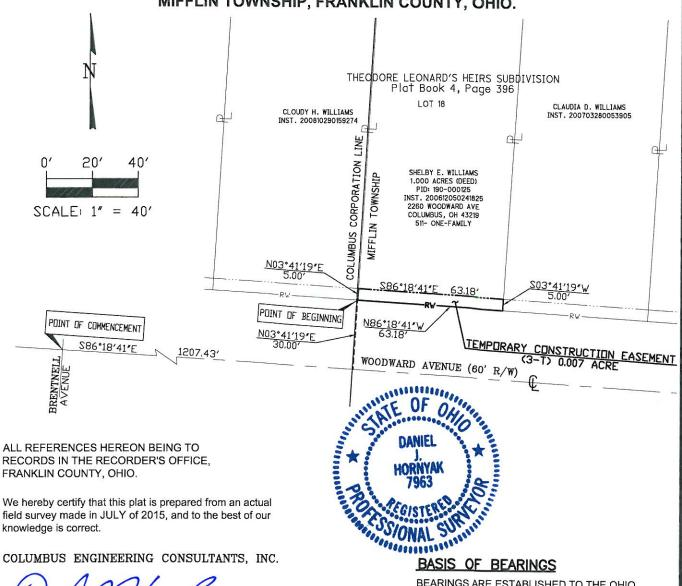
BEARINGS ARE ESTABLISHED TO THE OHIO STATE PLANE COORDINATE SYSTEM - SOUTH ZONE (NAD83) USING GPS OBSEVATIONS PERFORMED IN JULY 2015 WITH A BEARING OF S86°18'41"E ALONG THE CENTERLINE OF WOODWARD AVENUE, AND ALL OTHER BEARINGS CALCULATED FROM THIS MERIDIAN.
