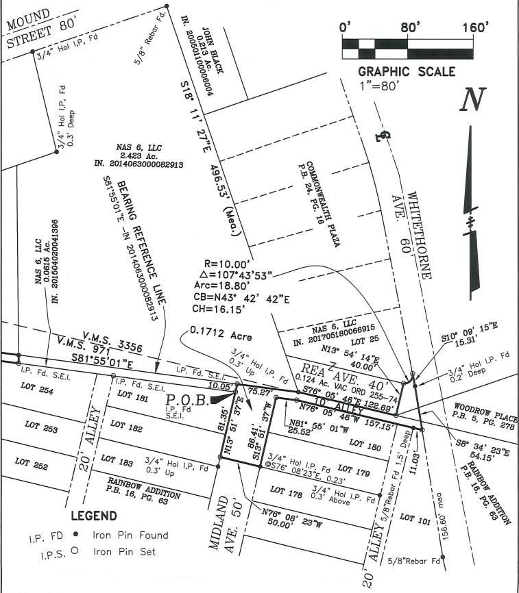
This plat was prepared from actual field survey during October 2018. Bearings are referenced to the south line of the 2.423 acre tract as called in Instrument No. 201406300082913. The iron pins set (I.P.S.) are 5/8" rebars, 30" long with yellow plastic caps stamped "SITE ENGLINC".
